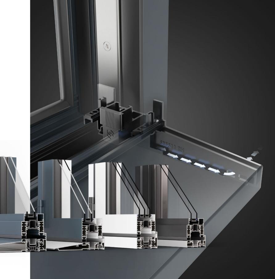
Prestige bi-folds come with four threshold options all featuring fully weather-sealed rebates that keep the worst of the British weather safely outside. These rebates also ensure doors aren't over-centred during operation, helping locks to engage correctly. Our doors also feature clever concealed drainage, eliminating the need for unsightly drainage cover caps.
